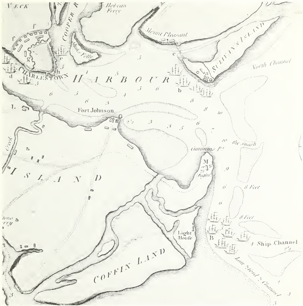
FIGURE 11.—Enlarged portion of Sayer and Bennett chart of Charleston Harbor (fig. 9), emphasizing the shoals at the entrance through which the deep-draft British frigates were forced to pass. Comparison of water depths with those of figure 10 shows a close agreement between these charts published respectively in England and America.
